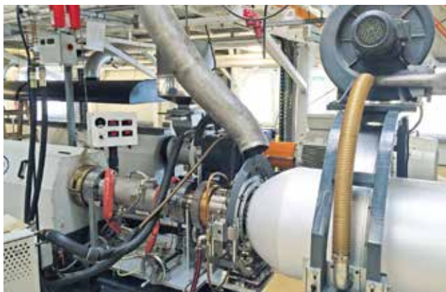
Fig. 5. Even lighter lightweight foam: A P1 cooling mixer integrated into the production of PS lightweight foam film improves cell structure and lowers the density (© Promix)
